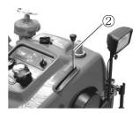
Operate the throttle dial to raise the pump pressure almost to 10 bar, and then check for water leaks from each part of the pump and the cooling water piping.
