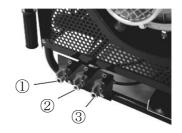
4. Insert the vinyl pipe in the container filled with anti-freezing fluid (180-200 mL).
