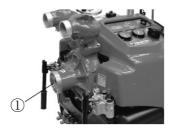
2. Pull the priming lever to run the primer, and check that the pressure gauge for suction pointer reads approximately -0.8 bar.
