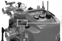
The pump identification number is marked on the pump casing.
