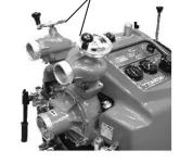
2. Start the engine, and pull priming lever ② to run the vacuum pump.
