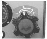
4. After a vacuum is produced, immediately return the priming lever to the original position, and stop the engine.
